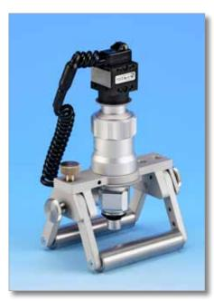
How can you get a four square meter workpiece under a metallurgic microscope? The solution to this problem is the Cellcheck CIL mobile USB measuring and inspection microscope. The Cellcheck CIL is always supplied with a stable MST stand. This allows secure positioning on flat material and on drums. The stand feet are coated
