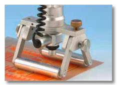
Lenses with magnification factors of 2x, 4x, 6x and 10x are included. The magnification factor based on a 17 inch PC monitor can be calculated by multiplying the magnification factor of the lens by 45. For example a 10x lens displays the measured point at a magnification of 450x. 15x, 20x and 30x lenses are available as options. A strong white LED provides coaxial illumination. The coaxially directed light eliminates all undesired reflections, which could lead to
